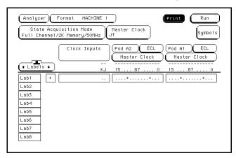
**c** Press the Trigger key. Make sure pattern term **a** is "A". If not, select the field next to "a" under the label Lab1. Type "A" then press the Select key.
